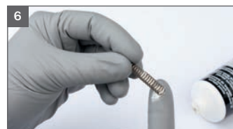
6 Grease and insert paint needle spring
