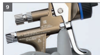
9 Grease visible part of air piston rod
