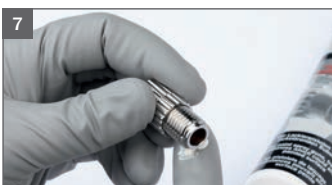
7 Grease thread of material flow control screw
